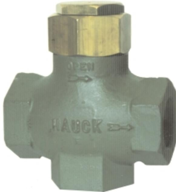
The Hauck LVG Series Limiting Orifice Gas Valves are designed to allow precise setting of high fire gas flow. They are used for single or multiple burner systems. The standard LVG series valves can be used as straight through type valves, and angle type valves are available to meet burner piping system requirements. These valves are designed for use with any commercial fuel gas; coke oven gas versions are also available.
