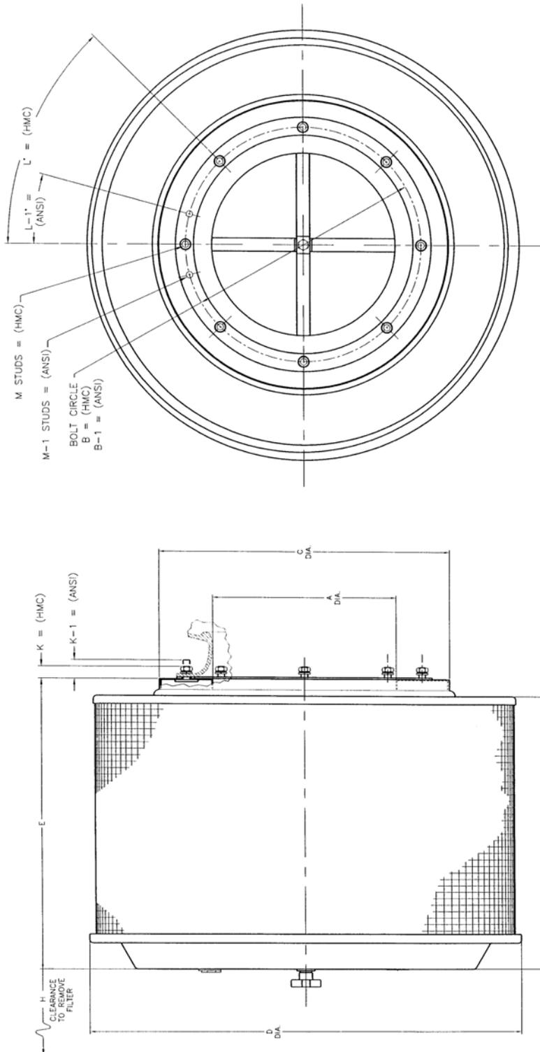
HMC = DIMENSIONS GIVEN FOR THE "HAUCK MFG CO." BLOWER INLET FLANGE (e.g. FBI1008-HMC). ANSI = CLASS 125 FLANGE CONNECTION, WITH STUD SIZE SHOWN, IS AVAILABLE WHERE APPLICABLE (e.g. FBI1000-ANSI). COMPLETE MODEL NUMBER MUST BE SPECIFIED ON ORDER.
