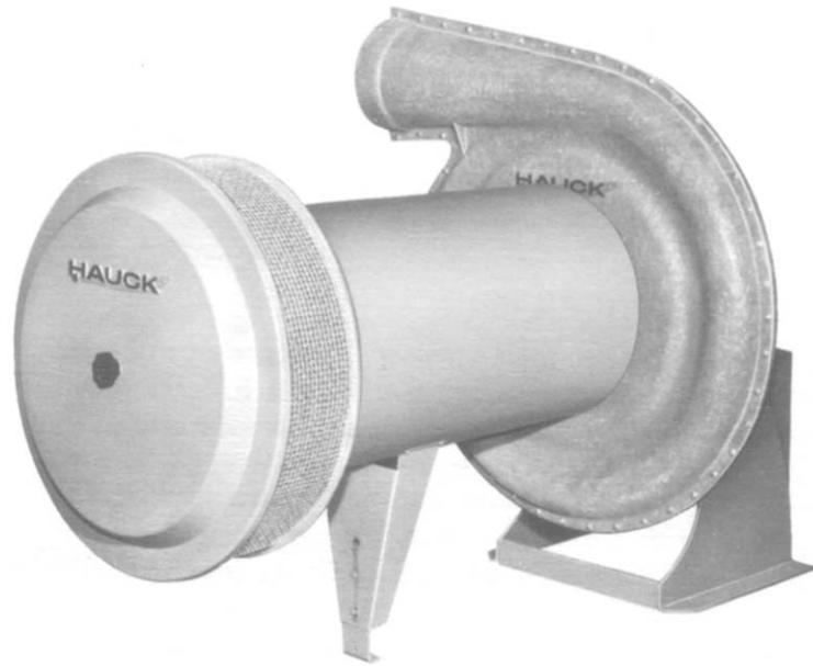
Hauck provides a complete line of highly efficient blower filters, silencers, and filter-silencers for use on TBA Turbo Blowers or any conventionally designed blower. These units offer not only efficient air filtration with a particulate removal efficiency of greater than 90% @ 10µm or larger, but also substantial reductions in dB(A) noise levels while making minimal demands on blower pressure.
