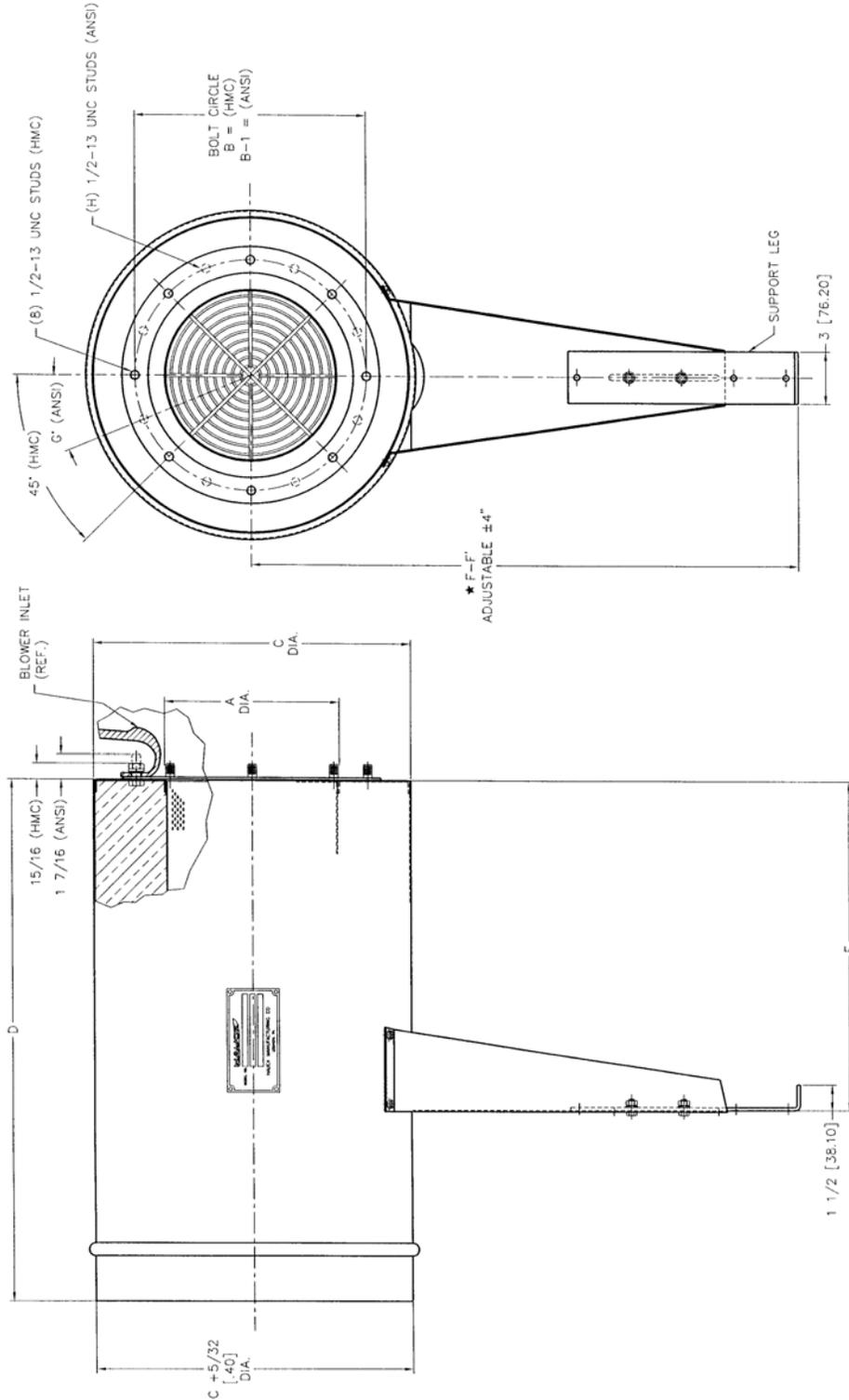
NOTE: DIMENSIONS GIVEN ARE FOR THE "HAUCK MFG. CO." BLOWER INLET FLANGE (e.g. SBI 2000-HMC). HMC = ANSI 125 CLASS FLANGE CONNECTION, WITH STUD SIZE SHOWN, IS AVAILABLE WHERE APPLICABLE. ANSI = (e.g. SBI 2000-ANSI). COMPLETE MODEL NUMBER MUST BE SPECIFIED ON ORDER.
