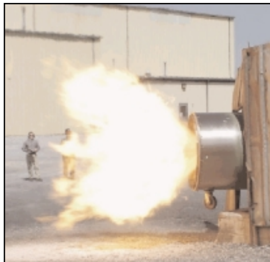
ECO-STAR II 150, 45 Spin, No. 2 Oil, 150 Million Btu/hr (44,000 kW)
