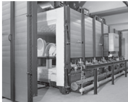
Intermittent shuttle kiln in the ceramics industry
