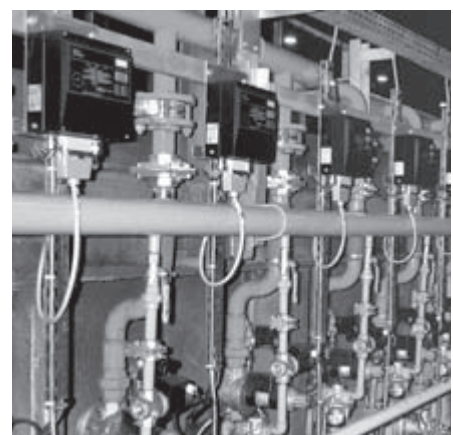
Hardening furnace with lots of industrial burners located side-by-side
