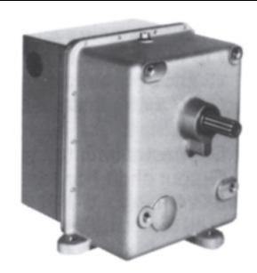
The EA-71 and EA-73 provide reliable performance for applications requiring high torque. The motors provide floating control via two 120VAC switched inputs. They include an integral 100-0hm slidewire for position feedback and a SPDT auxiliary switch. External current-toposition and resistance-to-position converters along with mounting brackets, linkage and associated components are available.
