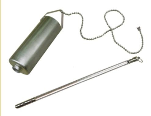
Hauck's Oil Viscometer Kit provides an easy, convenient and inexpensive way to rapidly determine the temperature to which oil should be heated to arrive at the proper viscosity for atomization. Kit includes viscometer and 0 - 300 °F scaled armor-cased thermometer.
